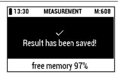
The save hint is shown only if memory space warning is on (see section 2.9.10, "Setting the memory capacity warning").
