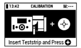
Insert the calibration strip of the recalibration set
