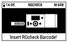
Remove the barcode strip for RQcheck from the pack. Insert the barcode all the way into the barcode reader in the direction of the arrow in a smooth motion from left to right, and then remove it again.
