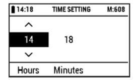
Select the desired time using the [Up] and [Down] buttons.
